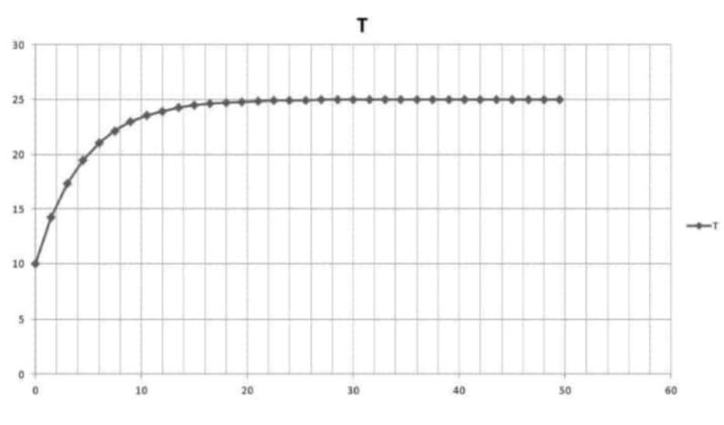
T-TAZCE T= 1A + Ce Kt T= 25-15e-0.222t ARM \$ 21->50 T = 25 - 15 \* exp (-0:222) \* + ) MATLAB simulation command windows close all Symst t2 0:05:50 T2 25.15 \* (exp(-0.222\* t)) I 2 Subs (7) Plot (t, To) & label (Time (min))) y label ('Temperature') axis tiglit gold on grid minor
