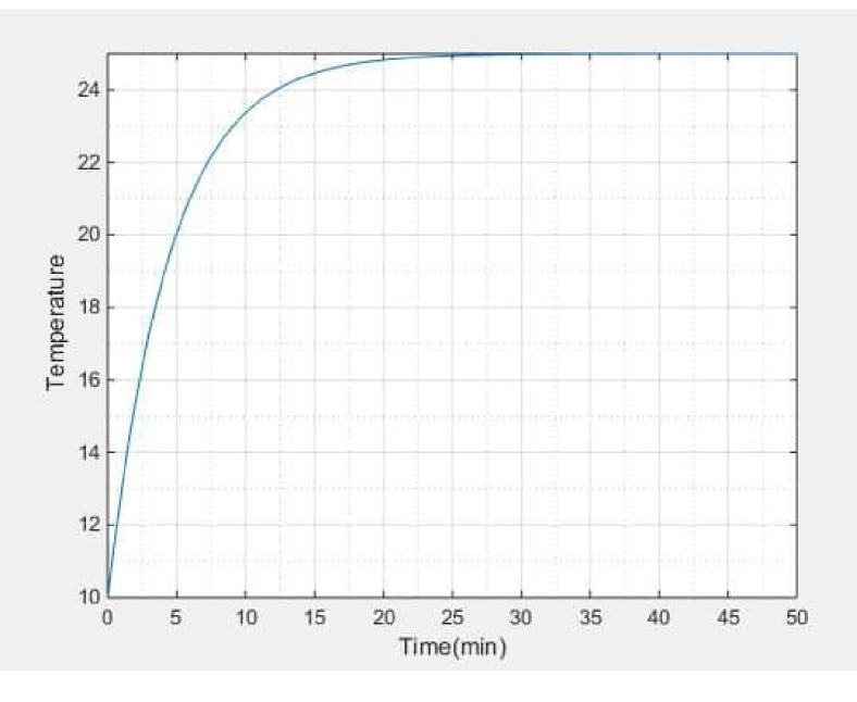
iv. The steady state temperature of the system is 25°C V. The system is not stable as the temperature changes with fine Vi We know that T=Ta+Clat
