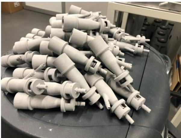
**figure 2. 1: 3D-printed Ventilators**
