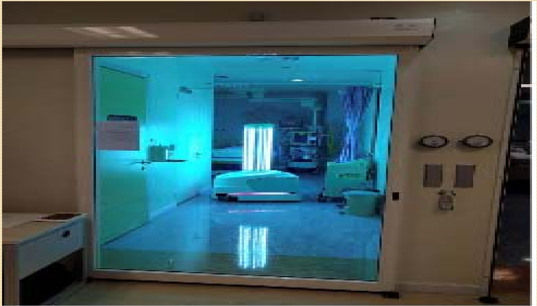
A UVD ROBOT DISINFECTING A MEDICAL WARD
