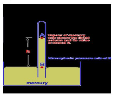
It is based on atmospheric pressure that acts on tube and retains mercury tube.
