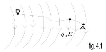
Consider the diagram above, suppose a test charge  $q_o$  is moved from point A to point B along an arbitrary path inside an electric field E. The electric field E exerts a force  $F=q_oE$  on the charge as shown in fig 3.1. To move the test charge from A to B at constant velocity, an external force of  $F=q_oE$  must act on the charge. Therefore, the elemental work done dW is given as:
