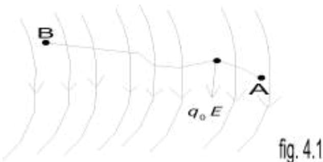
Consider the diagram above, suppose a test charge  $q_0$  is moved from point A to point B along an arbitrary path inside an electric field E. The electric field E exerts a force  $F = q_0 E$  on the charge as shown in fig 3.1. To move the test charge from A to B at constant velocity, an external force of  $F = -q_0 E$  must act on the charge. Therefore, the elemental work done  $dW$  is given as:
