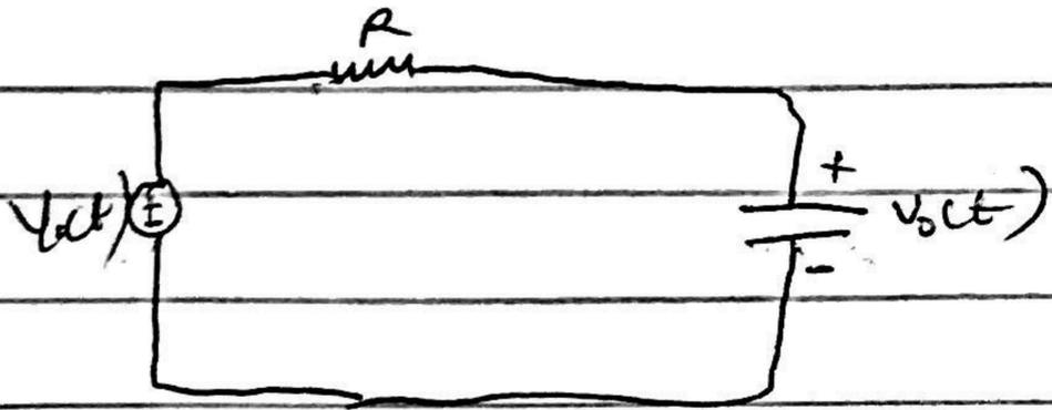
Fig Typical low-pass filter
