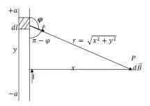
Fig 1: A section of a Straight Current Carrying Conductor Applying the Biot-Savart law, we find the magnitude of the field
