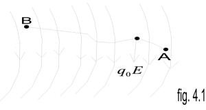
Consider the diagram above, suppose a test charge is moved from point to point along an arbitrary path inside an electric field. The electric field exerts a force on the charge as shown in fig 3.1. To move the test charge from to at constant velocity, an external force of must act on the charge. Therefore, the elemental work done is given as:
