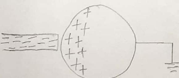
If the wire to ground is then removed, the conducting sphere is left with an excess of induced positive charge. Finally, when the rubber rod is removed from the vicinity of the sphere, the induced positive charge remains on the underground sphere and becomes uniformly distributed over the surface of the sphere.
