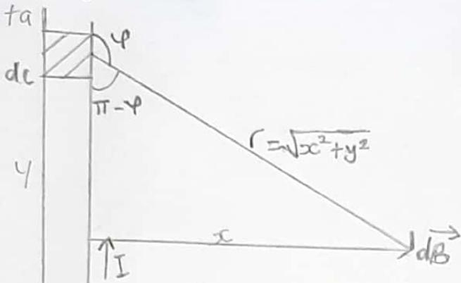
A section of a straight current carrying conductor
