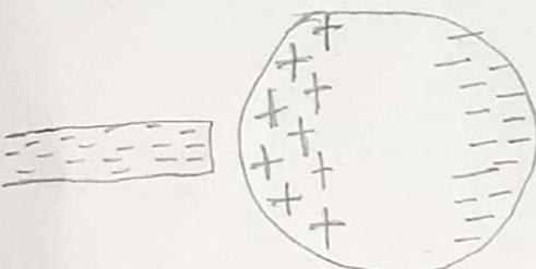
The region of the sphere nearest to the negatively charged rod has an excess of positive charge because of the migration of electrons away from this location. If a grounded conducting wire is then connected to the sphere, some of the electrons leave the sphere and travel to the earth.
