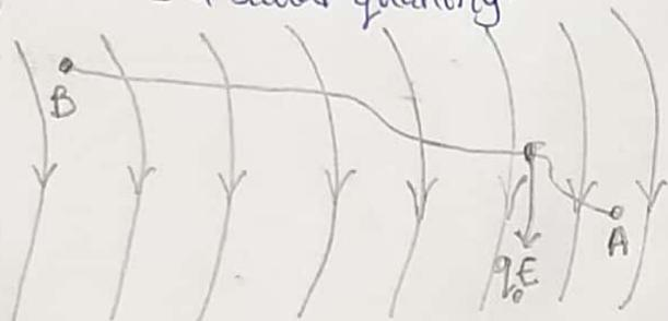
Consider the diagram above, suppose a test charge  $q_0$  is moved from point A to point B along an arbitrary path inside an electric field  $E$ . The electric field  $E$  exerts a force  $F = q_0 E$  on the charge as shown. To move the test charge from A to B at constant velocity, an external force of  $F = -q_0 E$  must act on the charge. Therefore the elemental workdone  $dW$  is given as:
