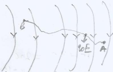
Consider the diagram above, suppose a test charge  $q_0$  is moved from point A to point B along an arbitrary path inside an electric field  $E$ . The electric field  $E$  exerts a force  $F = q_0E$  on the charge. To move the test charge from A to B at constant velocity, an external force of  $F = -q_0E$  must act on the charge. Therefore, the elemental work done  $dW =$
