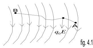
Consider the diagram above, suppose a test charge  $q_o$  is moved from point A to point B along an arbitrary path inside an electric field E. The electric field E exerts a force  $F=q_oE$  on the charge as shown in fig 3.1. To move the test charge from A to B at constant velocity, an external force of  $F=-q_oE$  must act on the charge. Therefore, the elemental work done dW is given as:
