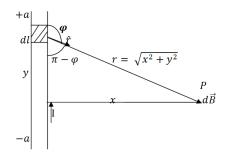
**5b.** Magnetic Field of a Straight Current Carrying Conductor
