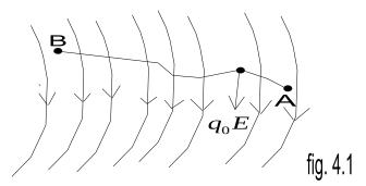
Consider the diagram above, suppose a test charge  $q_o$  is moved from point A to point B along an arbitrary path inside an electric field E. The electric field E exerts a force  $F = q_o E$  on the charge as shown in fig 3.1. To move the test charge from E to E at constant velocity, an external force of  $E = -q_o E$  must act on the charge. Therefore, the elemental work done E is given as:
