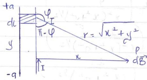
A section of a straight current-carrying conductor
