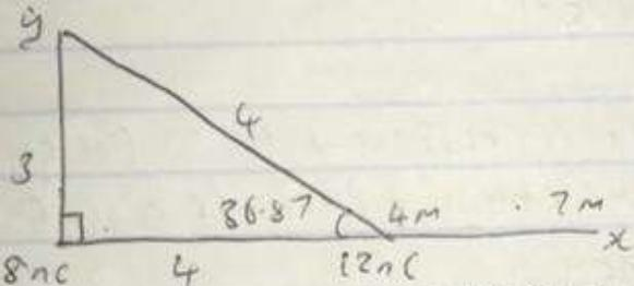
$$E_1(Q_1 \text{ to } P) = \frac{kq}{r^2} = \frac{9 \times 10^9 \times 8 \times 10^{-9}}{7^2} = 1.469 \text{ NC}^{-1}$$
