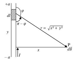
Applying the Biot – Savart Law, we can find the magnitude of the field  $d\vec{B}$   $B = \frac{\mu_0 I}{4\pi} \int_{-a}^{a} \frac{dl \sin \phi}{r^2}$  $\sin(\pi - \phi) = \sin \phi$
