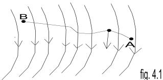
Consider the diagram above, suppose a test charge is moved from point to point along an arbitrary path inside an electric field. The electric field exerts a force on the charge as shown in fig 3.1. To move the test charge from to at constant velocity, an external force of must act on the charge. Therefore, the elemental work done is given as:
