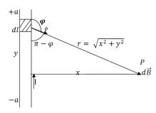
Fig 1: A section of a Straight Current Carrying Conductor Applying the Biot-Savart law, we find the magnitude of the field  $d\vec{B}$
