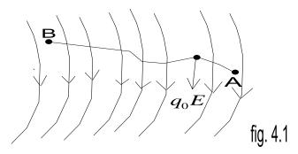
Consider the diagram above, suppose a test charge  $q_0$  is moved from point A to point B along an arbitrary path inside an electric field E. The electric field E exerts a force  $F = q_0 E$  on the charge as shown in fig 3.1. To move the test charge from E to E at constant velocity, an external force of E and E must act on the charge. Therefore, the elemental work done E0 is moved
