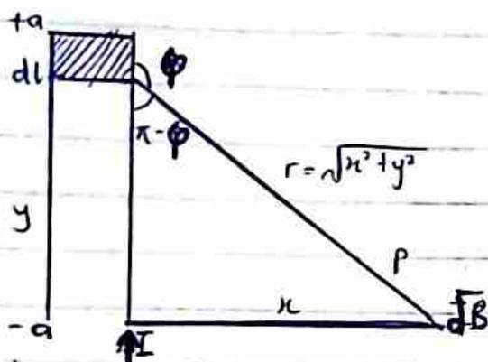
A section of a straight current carrying conductor
