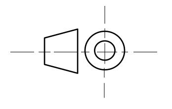
Third angle projection is that in which the object is placed below and behind the viewing planes, meaning it's plane of projection is placed between the observer and the object.
