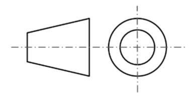
In 1st angle projection system, object is placed in the first quadrant and lies in between observer and plane of projection. In this object top view is drawn in the bottom of front view. And Left and right side views are drawn on right and left side of front view.
