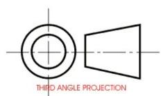
in third angle projection system the object placed in the
