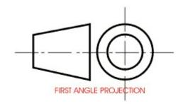
In the first angle projection system, the object placed in the first quadrant In 1st angle, the object is between the observer and the plane of projection,
