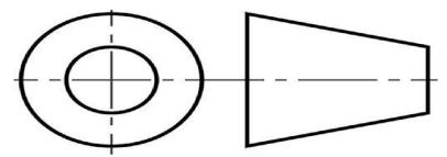
Third angle projection the object is placed below and behind the viewing planes
