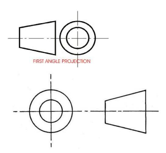
Third angle projection as seen above:in this method the projection plane comes in between the observer and the object.
