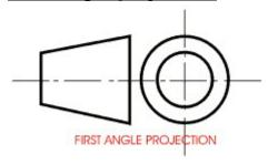
In the first angle projection system, the object placed in the first quadrant In 1st angle, the object is between the observer and the plane of projection,
