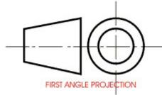
In the first angle projection system, the object placed in the first quadrant In 1st angle, the object is between the observer and the
