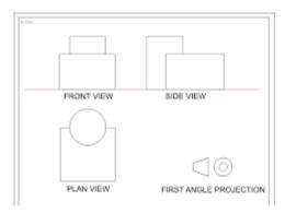
In the first angle projection system, the object placed in the first quadrant in 1st angle, the object is between the observer and the plane of projection.
