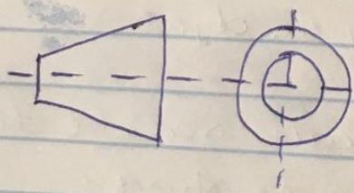
Third angle orthographic projection is a method of creating a 2D drawing of a 3D object with Front, Plan, and represented as
