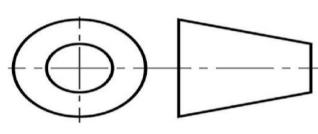
Third angle projection the object is placed below and behind the viewing planes meaning the plane of projection is between the observer and the object
