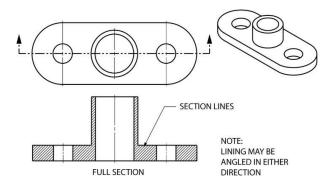
It is possible to section an object whenever a closer look intentionally is desired. Here is an object sectioned from two different directions.
