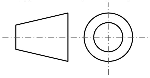
• Third angle projection the object is placed below and behind the viewing planes meaning the plane of projection is between the observer and the object.
