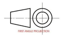
In the first angle projection system, the object placed in the first quadrant In 1st angle, the object is between the observer and the plane of projection,
