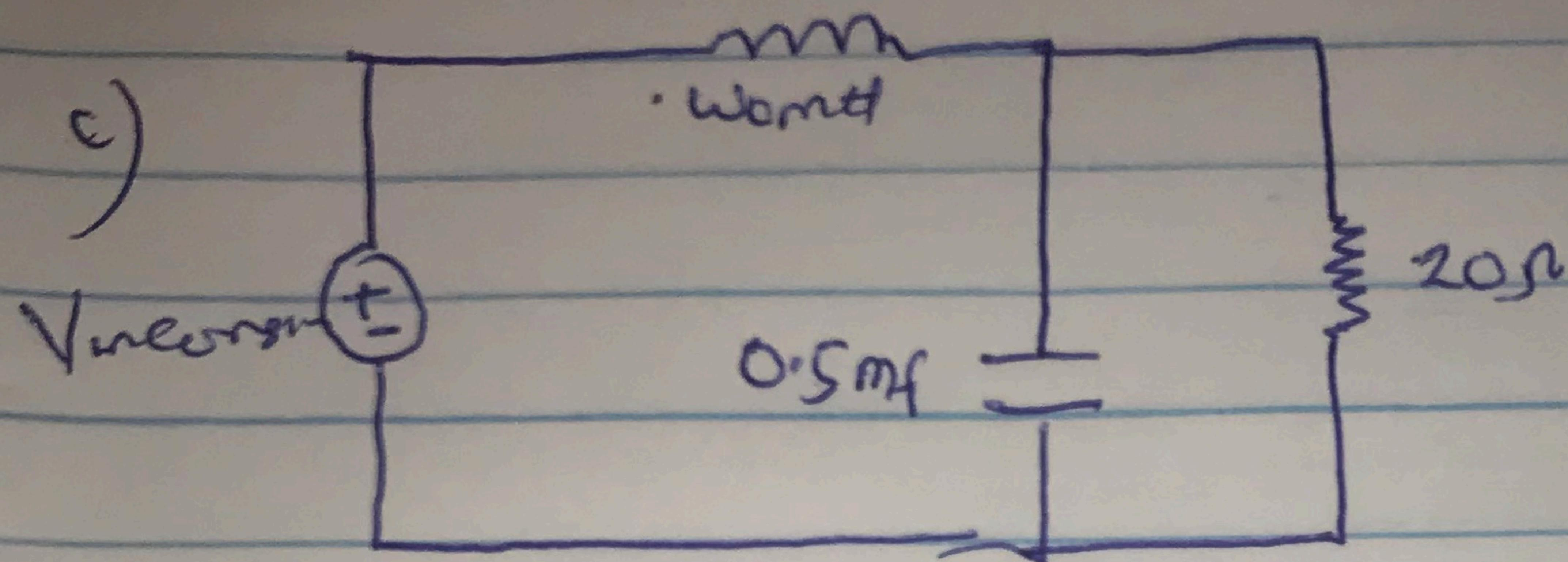
$$Z = j\omega(100 \times 10^{-3}) + \left( \frac{20}{j\omega(0.5 \times 10^{-3})} \right) \parallel \left( \frac{20 + 1}{1 + 0.5 \times 10^{-3}j\omega} \right)$$
