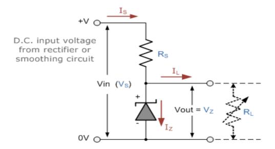
2.) A 5W maximum rated zener diode has 500mA maximum current flowing through it. If a 20Vmax bridge rectifier circuit is connected as input to the regulator circuit. Calculate:
