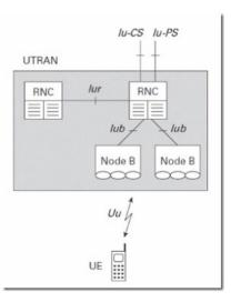
• NodeB: This is a physical unit for radio transmission and reception with cells. It may on or more cells depending on sectoring. It connects to the UE through the Uu interface.
