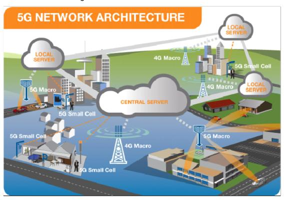
5G network architecture illustrating 5G and 4G working together, with central and local servers providing faster content to users and low latency applications.
