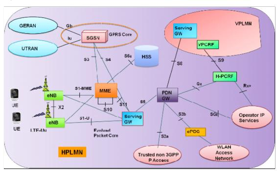
The figure above shows a Generic Mobile Communication architecture. 4G network is an integration of all heterogeneous wireless access network such as Ad-hoc, cellular, hotspot and satellite radio components. The technologies used in 4G are smart antennas for multiple input and multiple output (MIMO), IPv6, VoIP, OFDM and Software defined radio (SDR) System.
