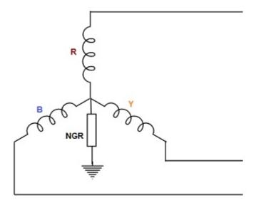
If there were no neutral, the voltage of the healthy phases would have been increased during the ground fault, which may eventually lead to insulation failure of the healthy phases. Thus a single line to ground fault may result in three phase fault due to insulation failure.
