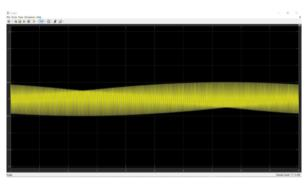
E. When the signal of 2K ohms is passed through the filter, the following will be obtained. The transfer function equation for the circuit is given below as (1/RC)/(S + 1/RC)When R= 2,000 $\Omega$  and C= 0.01F Transfer Fcn = (1/2000\*0.01)/(S +(2000\*0.01)) = (0.05)/(s+0.05) therefore:
