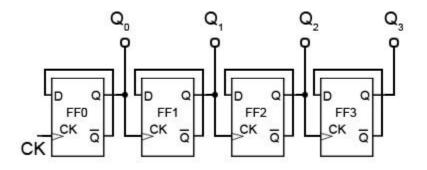
A 4 bit asynchronous DOWN counter is shown in above diagram. It is simple modification of the UP counter. 4 bit DOWN counter will count numbers from 15 to 0, downwards.
