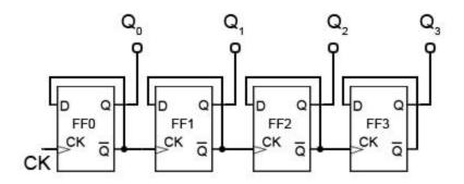
A 4 bit asynchronous UP counter with D flip flop is shown in above diagram. It is capable of counting numbers from 0 to 15.
