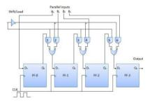
**Parallel Input Parallel Output (PIPO):** In this mode, the 4-bit binary input B0, B1, B2, B3 is applied to the data inputs D0, D1, D2, D3respectively of the four flip-flops. As soon as a negative clock edge is applied, the input binary bits will be loaded into the flip-flops simultaneously. The loaded bits will appear simultaneously to the output side. Only clock pulse is essential to load all the bits.
