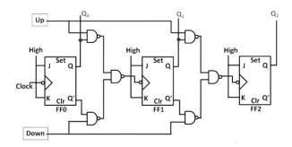
**UP Counting:** If the UP input and down inputs are 1 and 0 respectively, then the NAND gates between first flip flop to third flip flop will pass the non-inverted output of FF 0 to the clock input of FF 1.
