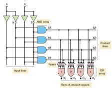
A device that be programmed by blowing the appropriate fuses at the input to the OR array
