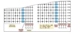
**Programmable array logic (PAL):** Every AND gate can be programmed to generate any desired product of four input variables. The PAL family also contains devices with variations of the basic SOP circuitry. Channel SOP logic circuit to a D FF input and use one of the pins as a clock input, to clock all of the output flip-flops synchronously. These devices are referred to as *registered PLDs* because the outputs pass through a register.
