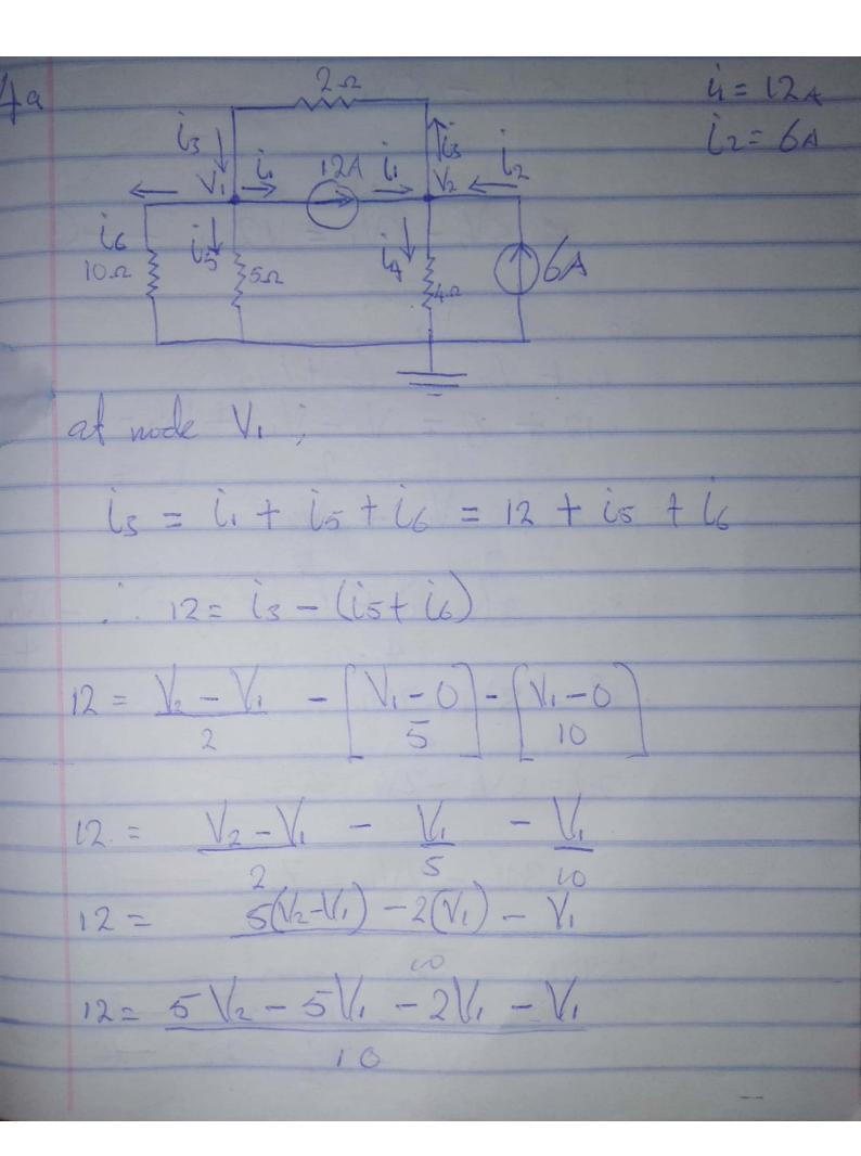
12: 5 V2 - 8 V1 18 5/2-8V1=120 -- C at node V2; i. i. + iz = is + i4 1.12+6= V2-V1+ (V2-0) 18 = V2 - V1 + V2 18 = 2 (V2-V1) + V2 = 21/2-21/11/2 18=31/2-2VI 72= 3 /h - 2/1 - 3 V2 - 2 V1 = 72 Solving Simultaneously 542 - 841 = 120 -(2) 3V2 - 2V1 = 72
