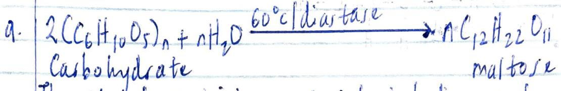
The starch containing materials including molasses, potatoes, cereals, rice and on warming with malt to 60°C for a specific period of time are converted into maltose by the enzyme diastase contained in the malt.
