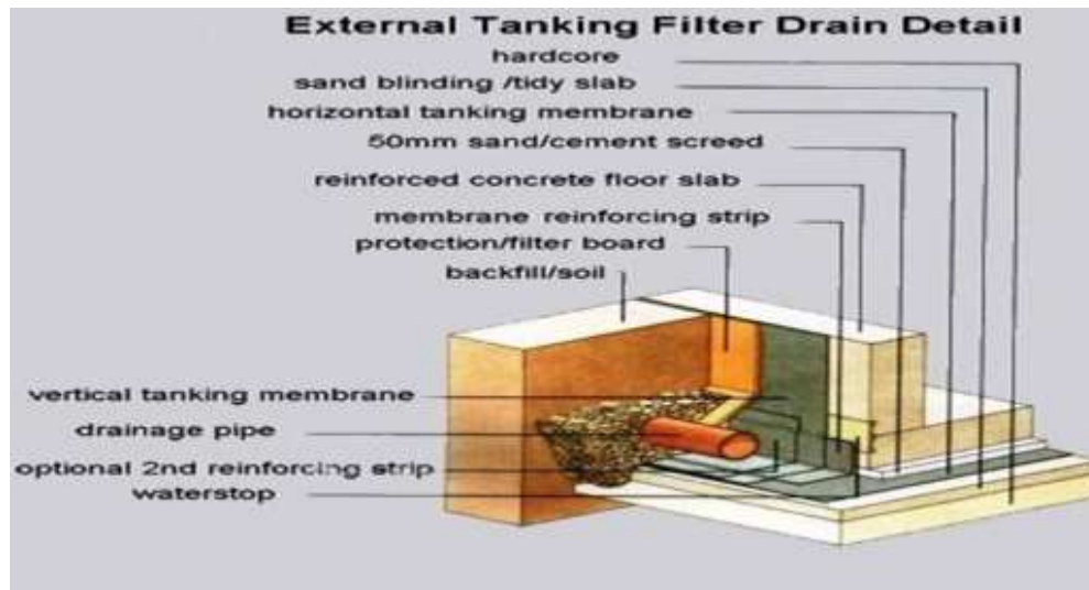
Figure 1: External Tanking System.
