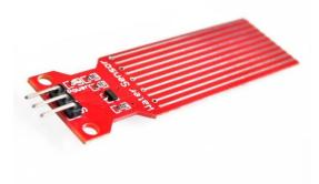
Rain Sensor, is one kind of switching device which is used to detect the rainfall. It works like a switch and the working principle of this sensor is, whenever there is rain, the switch will be normally closed.
