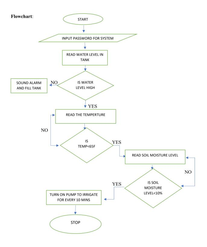
**Implementation**: the application software can be implemented using the algorithm above with various programming languages. Bearing in mind that the application software should be able to interact with machine, some hardware parts of the machine would have to be changed or upgraded. It would most likely be implemented using ARDUINO or Raspberry Pi with high level programming languages like PYTHON, java, etc.
