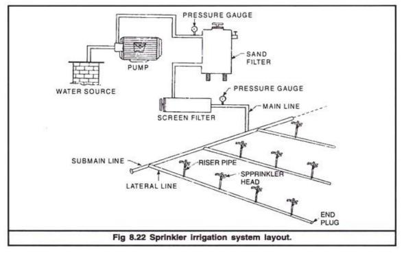
The pump unit is usually a centrifugal pump which takes water from the source and provides adequate pressure for delivery into the pipe system.
