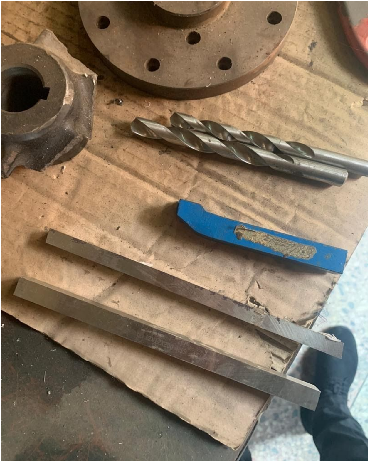
Figure 3.7: Hss tool, carbide turning tool and drill bit
