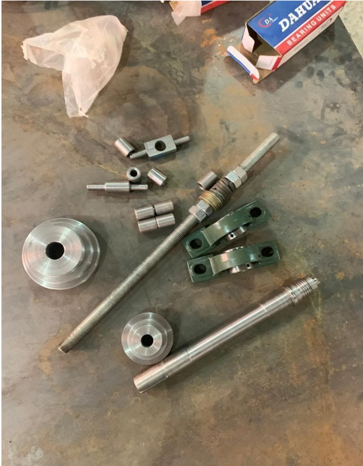
Figure 3.1: Components of head stock before assembly
