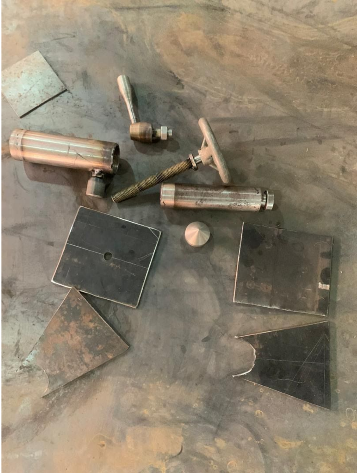
Figure 3.3: Components of tail stock before assembly
