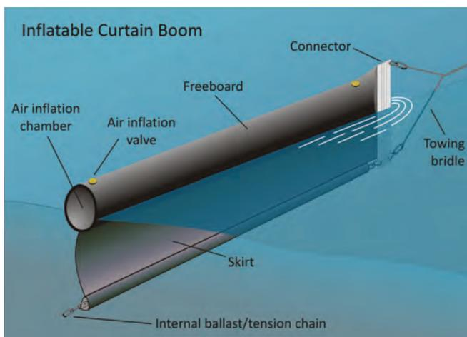
▲ Figure 2c: An inflatable curtain boom with a combined ballast and tension chain fitted in an integral pocket attached to the bottom of the skirt.
