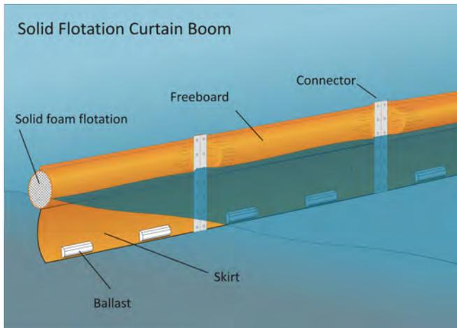
▲ Figure 2a: A solid flotation curtain boom with external ballast.
