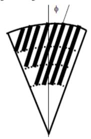
Bar edge length is the total length of bar edges that the fibres will see in one revolution. Note that for a double
