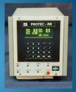
A microprocessor-based digital protection relay can replace the functions of many discrete electromechanical instruments
