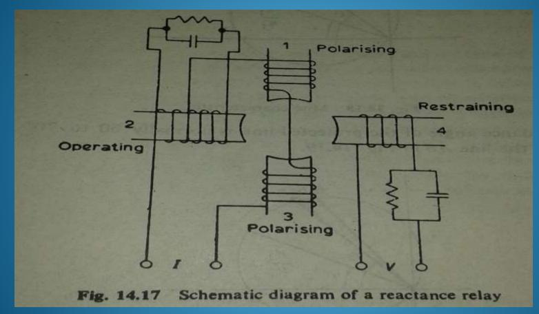
It is a four pole structure. This has operating, polarising and restraining coils.
