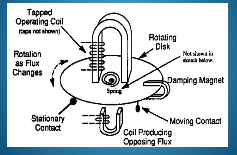
•An induction relay works only with the alternating current.
